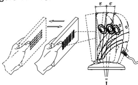
**Figure 11 - scanner position adjustment**
